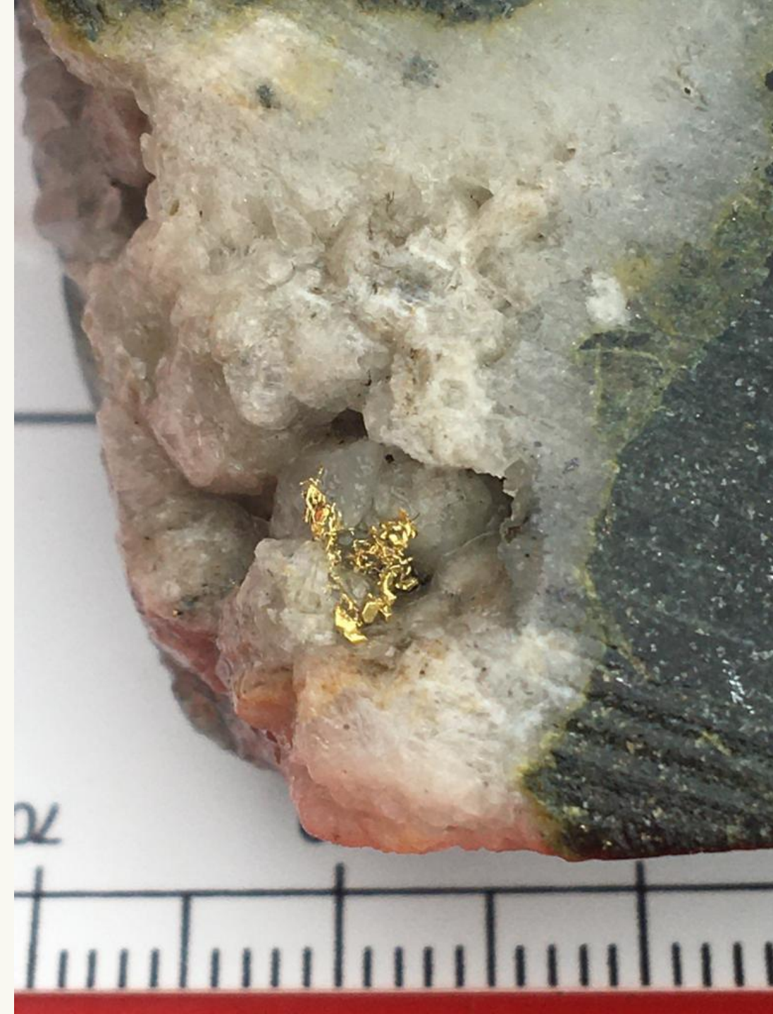
Image: QM-DH-34, 268.5m. Coarse grain dendritic gold in quartz-carbonate cement.
