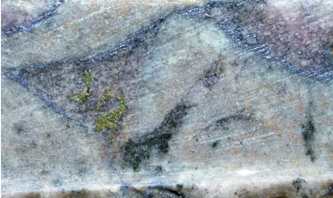
Figure 3: Los Calatos diamond drill core showing the presence of copper and molybdenum
