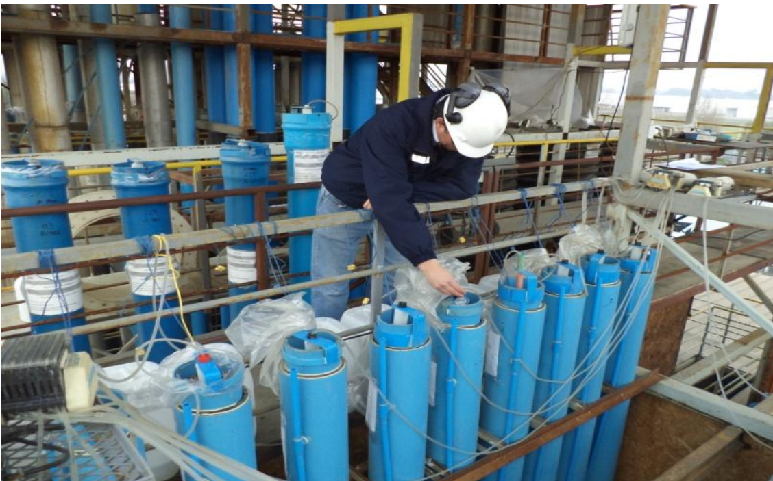
Figure 8: Checking the flow rates at the top of the 6 metre columns, SGS laboratory, Santiago, Chile.
