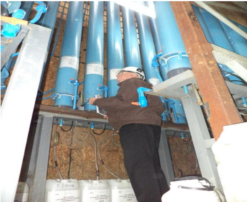
Figure 8: Checking the flow rates at the top of the 6 metre columns, SGS laboratory, Santiago, Chile.
