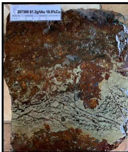
Photos: Left- Initiating the extension trench at Leah's Lode. Right- Polished outcrop sample of garnet-chalcopyrite skarn grading 61.3g/t Au and 18% Cu 1 taken ~2m from the original Leah's Lode trench.
