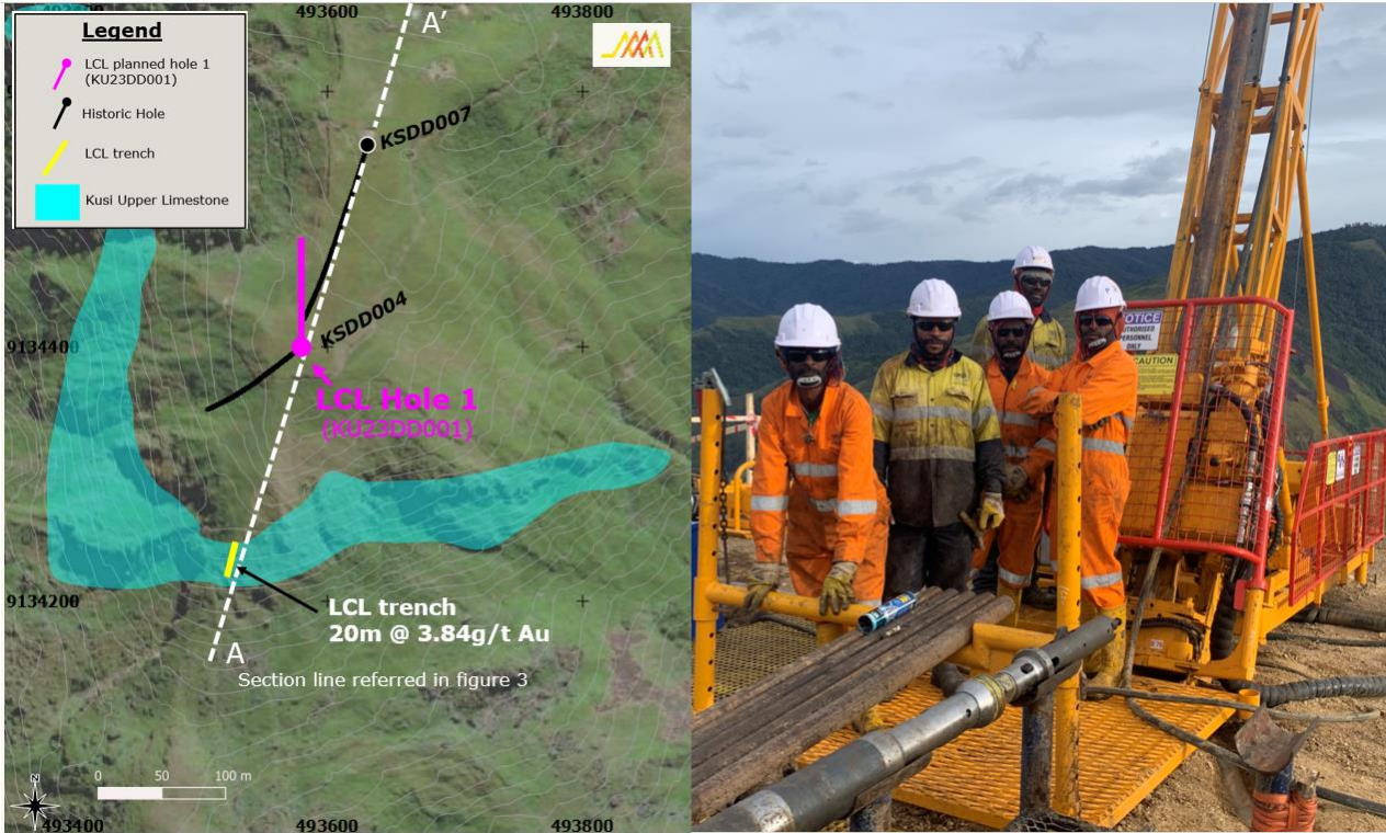
Figure 2: Plan view of current drill hole with historic drill hole traces, "Upper Limestone" unit with LCL trench location. Photo: QED drilling team at LCL hole 1.
