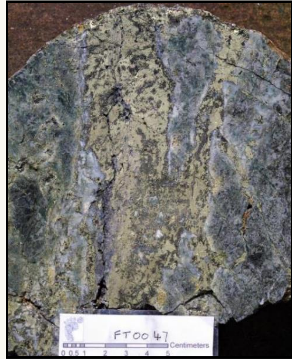
Copper/gold polished sample from Ubei Target. Chalcopyrite-silica-arsenopyrite-pyrite. 9.5% Cu, 156g/t Au Sample 0047
