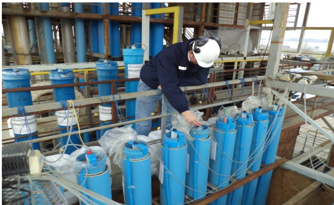
Checking the flow rates at the top of the 6 metre columns, SGS laboratory, Santiago, Chile.
