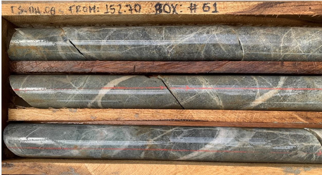
Photo 1: Drill core from TS-DH08. The mineralised rock of the cupola is typical medium-grained diorite with moderate potassic alteration and porphyry style A-type veinlets (2-10mm; 10-15/m) (thickness; density), disseminated pyrite and magnetite and overprinted epithermal style ISS veinlets (3-5mm; 3-8/m) (see also Table 1, attached).
