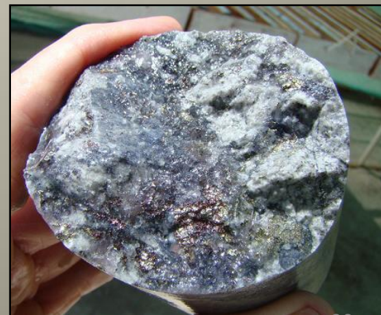
Primary Cu-Mo mineralisation in drill core
