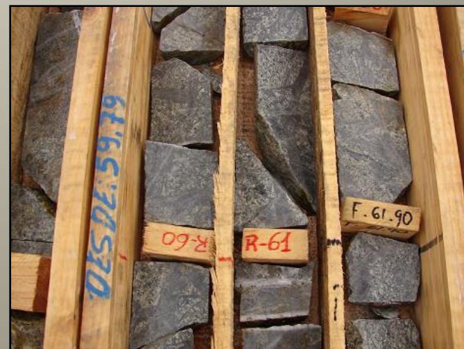
RIGHT: Supergene mineralisation (hole MD08)
